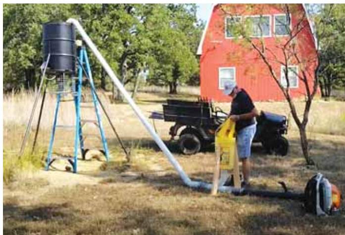
Curved leg of a pvc Y joint is attached beneath a hole in the bottom of the bucket. The straight leg of the joint is attached to the leaf blower tube with a flexible connector.
