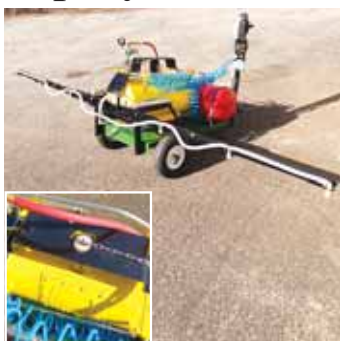
Liquid tank can’t be pressurized unless the filler plug is locked in, and the iron lock is over the top of the plug.
