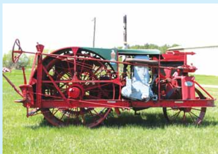
Case 10-20 is powered by a 4-cyl. gas engine, the same one used in Case automobiles at the time.
