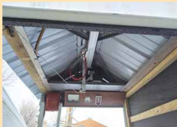
Interior view of carriage, which can carry up to 400 lbs.
