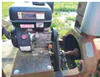
Predator 212cc engine has 6.5 hp. and runs at 3,600 rpm's.
