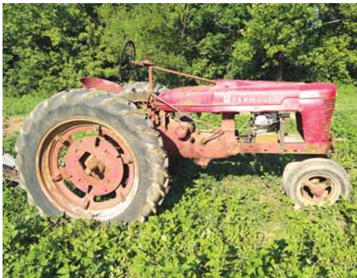
1941 Farmall H repowered with a Predator 212cc engine.
