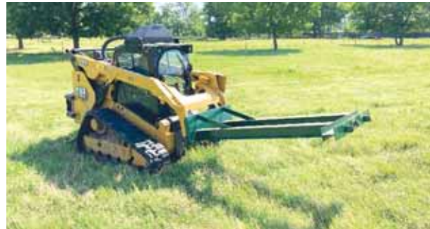
Mound pusher built from a 5-in. I-beam can reach under fences.
