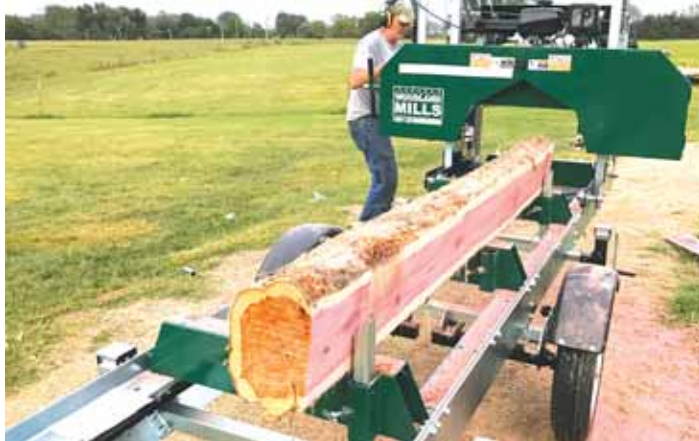
All three models share a 4-post head design with a tubular back beam for rigidity to provide smooth and accurate cuts. The head moves up and down galvanized steel posts via a hand crank system.
