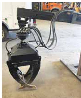
Claw was developed by county highway department workers to clear dams.
