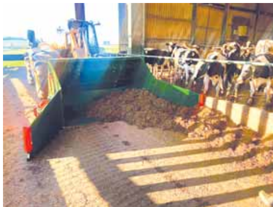
Side panels on the buckets open and close hydraulically and can be adjusted on the go. A bright orange tube on the end of panels is a replaceable steel wear part.
