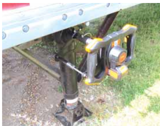
Lift tool raises and lowers trailers and grain hoppers using a battery.
