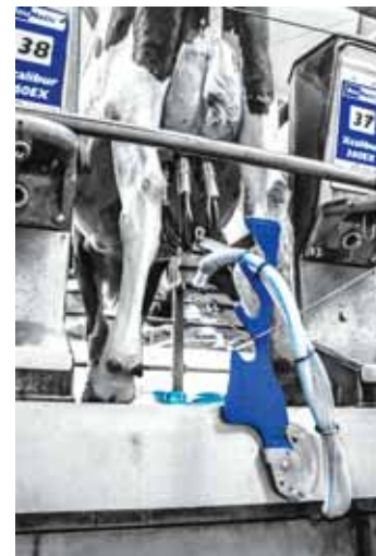
Metcalfe credits a local design and fabrication firm with helping him develop Lactalign. The device evens out the weight distribution of the cluster across the four quarters.
