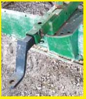
I got tired of having to unhook the blade behind my tractor whenever I wanted to tow a wagon. So, I welded a 2-in. receiver hitch to the top of the blade and now I just insert a ball hitch or flat hitch into the sleeve when I need to pull something. (Bill Stowe, Essex, Ontario)
