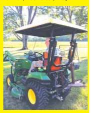
I made a canopy to fit my Deere 1023 garden tractor using the top of an old combine cab. I bought metal to make the mounting brackets and carefully welded them to just the right angle so the top would be level. It took a while to get it right but now I'm mowing in the shade all the time. (Jack Suits, 250 N Jefferson St., Wabash, Ind. 46992; ph 812-216-0840)
