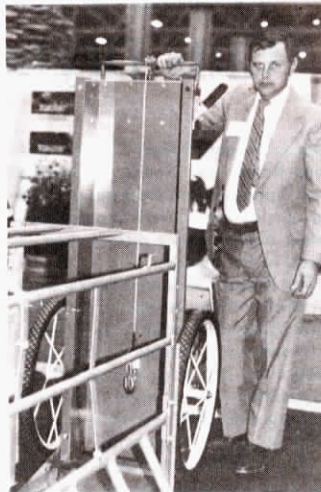
Dick Eklund demonstrates how cart tips vertically for loading dead sow out of crate.
