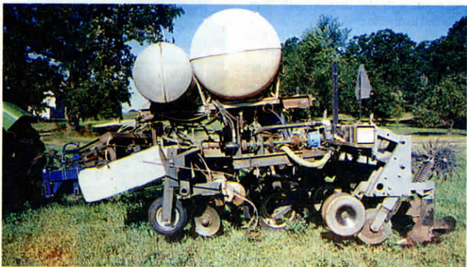
He removed the Hiniker cultivator's disc hillers and mounted them up front away from the sweeps to improve trash clearance.
