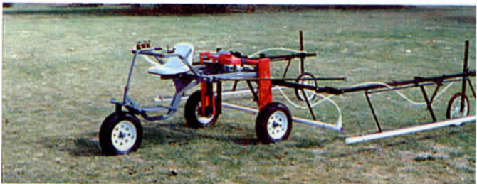
A 30 1/2-ft. wide, 3-section Speidel applicator mounts on a 3-wheeled Nitzsche self-propelled weeder.
