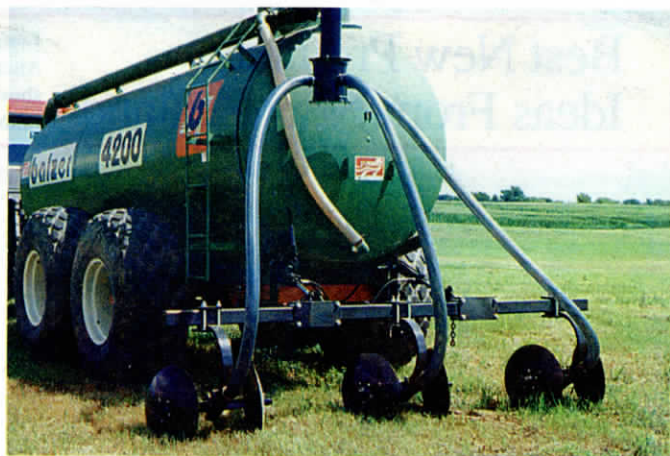
Applicator has three pairs of coulters, with each pair mounted on a single shank that clamps onto toolbar. Manure is delivered through hoses behind each shank.
