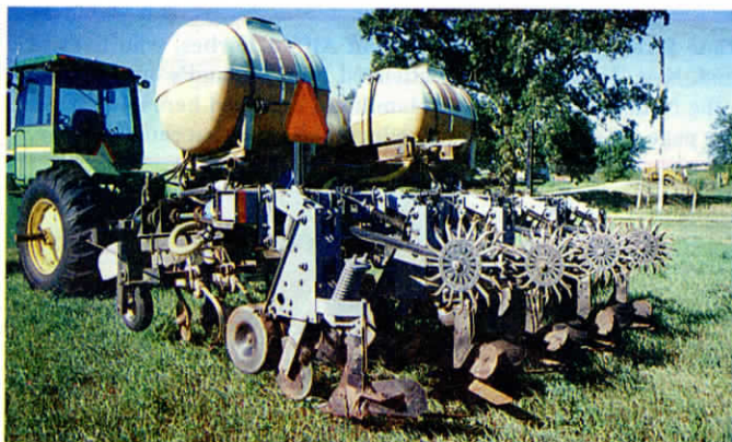
Peterson built the cultivator out of a Blu-Jet caddy, Orthman guidance system, and Hiniker cultivator. He uses a Deere 8430 200 hp tractor to pull it.
