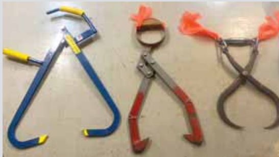
Tierney’s log handling tools include Pinch-A-Log (left), a set that he made himself (center), and his favorite set that was made in the early 1900’s.
