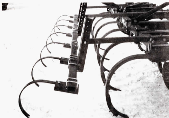
Most owners equip rear-mounted leveler attachment with 7 in. sweeps. They're spaced 1 ft. apart (1.5 ft. apart on 3 bar chisel plow) and are set to run about 4 in. deep.
