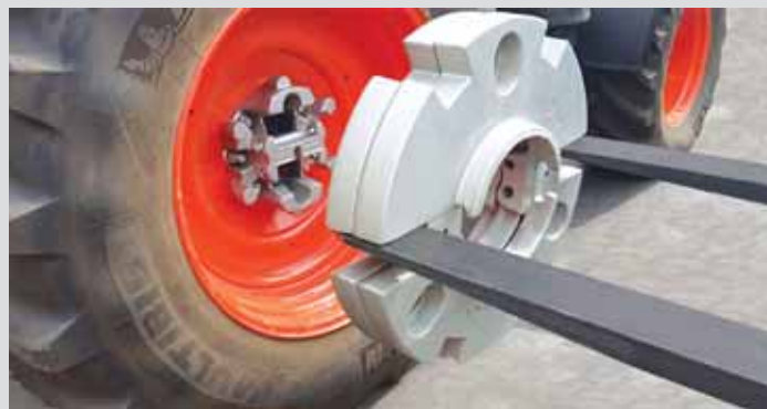
Easymass wheel ballasts are lifted in place with a forklift for easy mounting.
