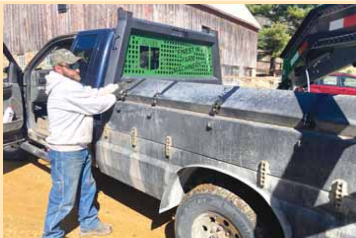
Jacobson shows his roller chain hinges on his pickup box.
