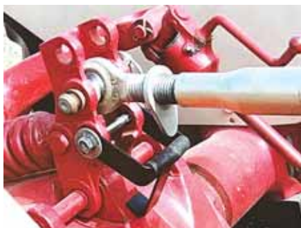
Chicklo says it's easier to hook up implements to his Ford 8N after he made this simple bumper bracket to keep the top link away from the pto.
