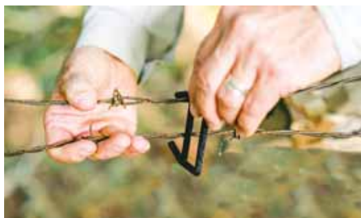
Wire-Ups hold barbed wires together so people can crawl through a wider opening without damaging clothing or gear.
