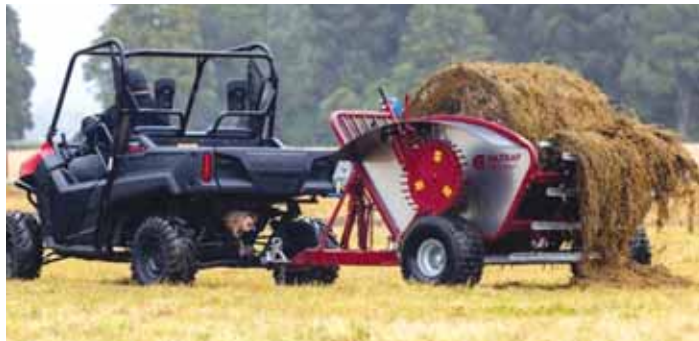
Ellis Bale Buggy works behind an ATV, UTV, pickup, or horse and is ground-driven.
