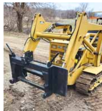
Carolla attaches his 3-pt. Quick Hitch plate to the skid steer mounts he made for his Magnatrac.
