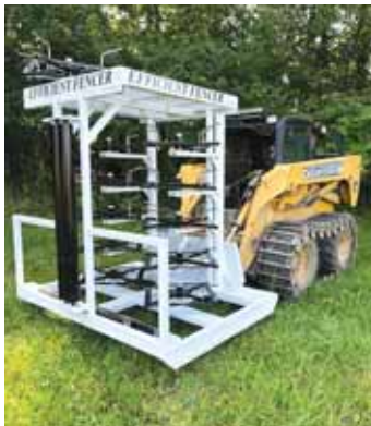
Fencer has multiple de-reelers which swing out for reloading.
