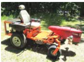
Clifford's custom runaround cart has several different attachments like a David Bradley hood (above) and a hydraulic dump cart (below).
