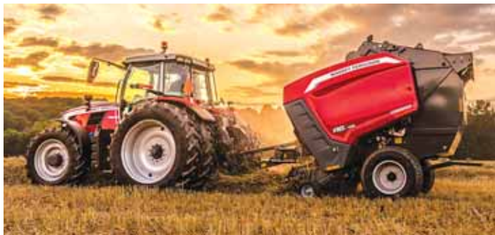
RB.156 new features include a camless pickup, a new front rotor that runs counter-clockwise, and a retractable floor bottom.
