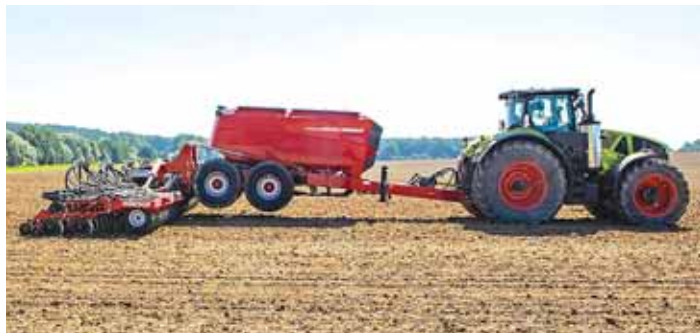
Planter adjustments are made by deactivating and hydraulically lifting every second row.
