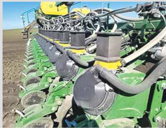
Ehlers has made his own replacement parts using a 3D printer, saving time and money.
