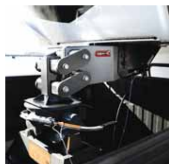
Gen-Y Hitch automatically latches when you drop it over the ball as well as unlatches from the outside of the truck bed by using a hook or rope.
