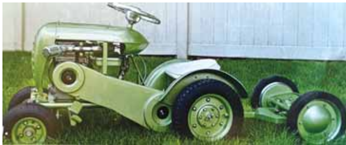
Matt Castagno converted an antique push-type reel mower into a pull-type model for his custom-built tractor.
