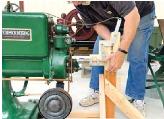
Miller's design allows him to start his hit-and-miss engines by himself.
