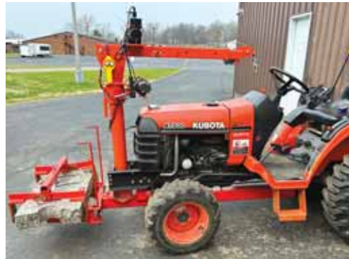
Hoist's boom swings right and left to put the stone in place and can also be flipped back over the cab and secured in place when not needed.
