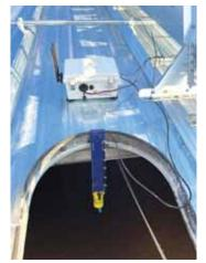
Unique sensors read CO2 levels each hour. Normal readings are between 300 and 500 ppm, but if over 1,000 ppm, the grain is beginning to spoil, or large numbers of insects are gathering and eating.
