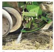
Tiny trench created by the jets offers the proper seed placement depth with minimal spray or dust back.
