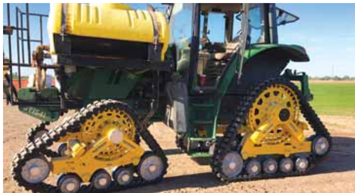
"We had to design a tread that could handle the narrower road wheels and still carry the load," says Laux.
