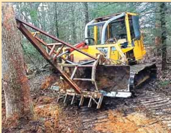
Mike Belben built a multi-purpose tree spear and root digger he mounted on the blade of his dozer.
