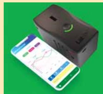
Labby, Inc. is producing handheld and inline automatic milk quality testing equipment that uploads data so producers can view results on a smartphone app.
