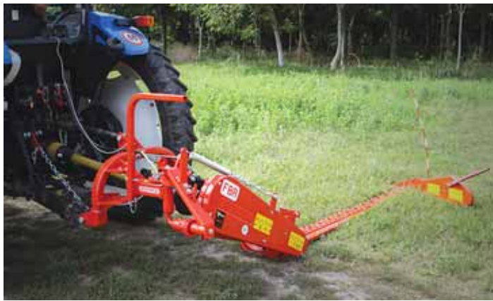
What sets the Fiore model apart from other sickle mowers are its anti-vibration features and double action—both the sections and the guards move.
