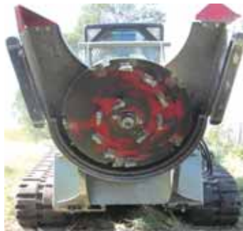
Grinder saw cuts trees up to 6 in. in dia., which can then grind the stump as well.
