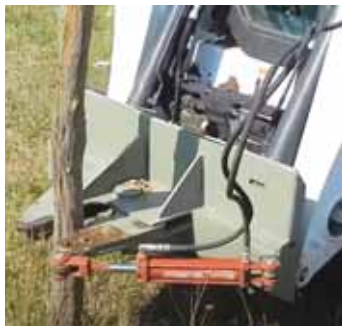
Post-puller has sawtooth edges that grip posts for easy removal.
