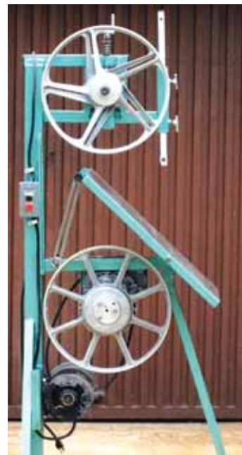
Drive wheels on Tony Foale's shop-built bandsaw are from discarded moped wheels.
