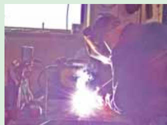
Welder runs on four batteries and can last long enough for remote repairs.
