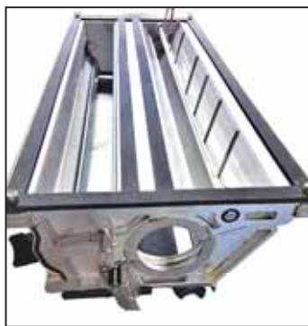
The meter boxes fit the John Deere 1900 and 1910 series carts along with those built by Flexi Coil and Case New Holland.
