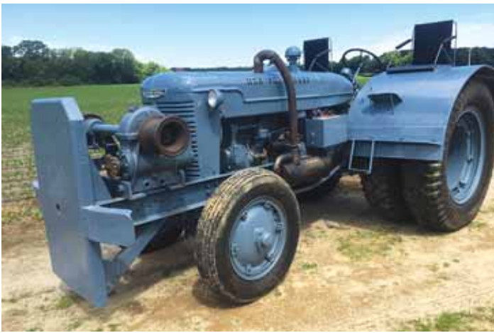
Garrison "Doc" Brown restored this rare 1943 model International Harvester I-9 Special to its "like new" condition. Painted Air Force blue, the I-9 was used by the military during WWII for towing vehicles, supplies, and explosives.
