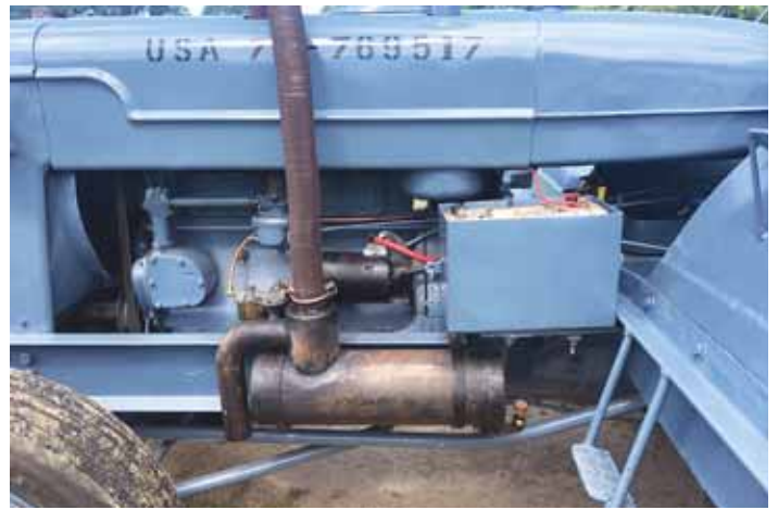
Exhaust system has a water bath to capture sparks because the tractor towed equipment carrying explosives.
