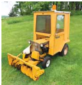
Allis-Chalmers mounted a prototype cab on a Big 10 lawn tractor in the 1960s.
