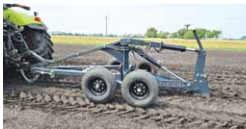
Hydraulics control both depth and pitch to create a long-lasting and open channel.
