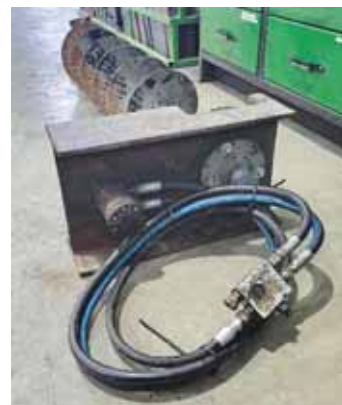
"I had a chunk of I-beam left over from when I built my house, which made the main frame," Madsen explains. "The hydraulic motor and hoses came off an old bin sweep that hadn't been used for years, while the gears are off an old swing-away auger that rusted. I dismantled it for the steel and a few parts."
