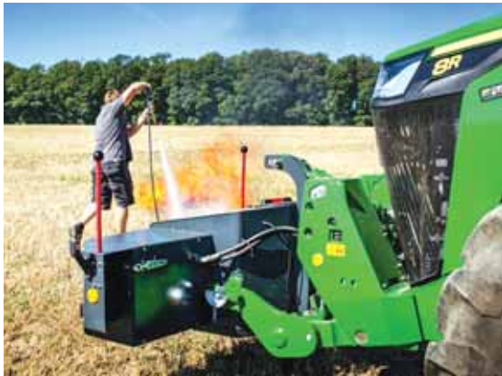
Field Attack provides up to 13 min. of water at pressure to extinguish fires.
