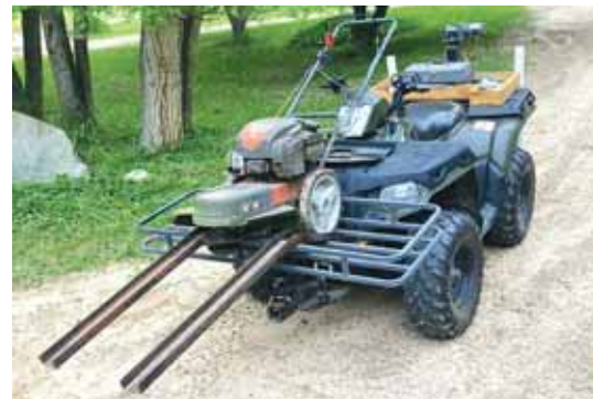
“The forward end of the tracks rest on the ground until I push the trimmer up and onto the cargo carrier,” says Sieting. “As I do that, they rock up and out of the way as I drive.”
