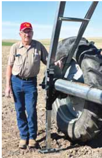
Pivot Jack has a 7,000 lb. capacity and an infinite height tolerance, which allows for greater precision.
