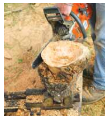
"Thickness is crucial, and I've learned how to watch the blade," Henry says. His goal is to saw the wood down to 1/2 in. thick or less and to keep the depth fairly uniform.
