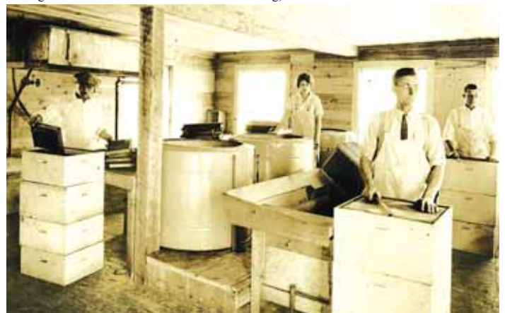
Honey was extracted from hives on the upper level of the barn and flowed to packaging on the lower level.
