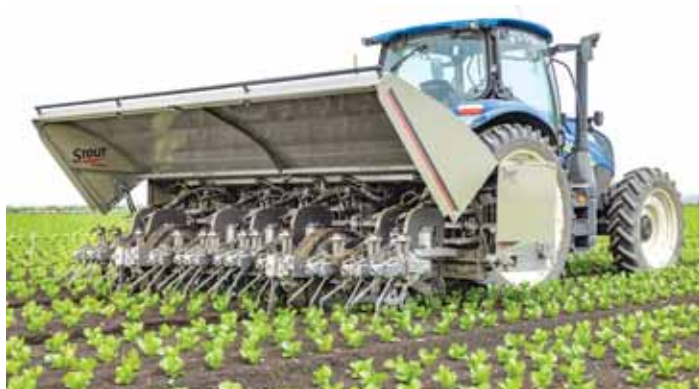
Six-row Smart Cultivator uses its machine vision and artificial intelligence to cultivate and weed using mechanical blades. The software ensures accuracy to 99 percent.
