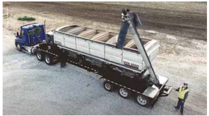
Heartland Ag Tender auger rotates 270 degrees.
