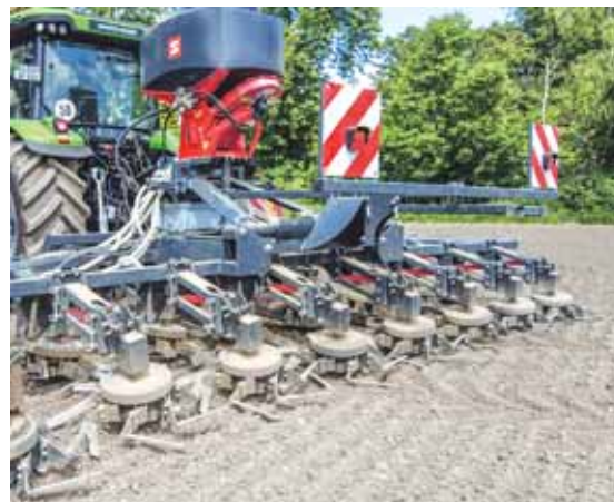
A key feature that caught farmer interest is the parallellogram-guided suspension of the tools. According to product manager Ole Denker, this ensures uniformly shallow processing.
