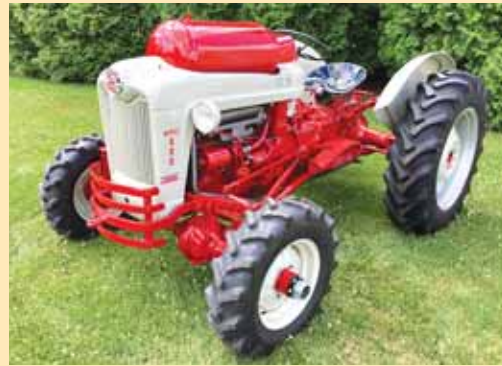
1955 model 650 restored by adding a Sherman-NAPCO front wheel drive and an LP kit.
