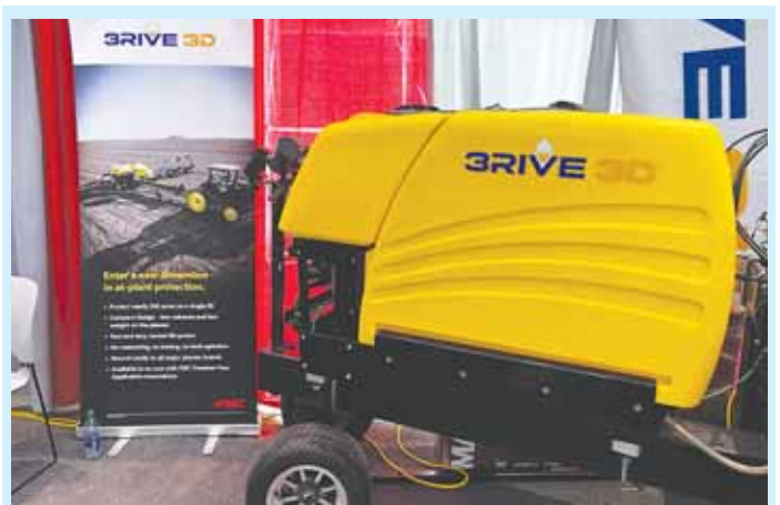
The solution expands 50 times as it mixes before being delivered to row units, and using air as a carrier reduces water use by 90 percent in a traditional liquid system.
