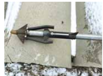
Grapple shown folded flat to drive through blockage.
