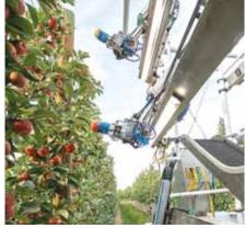
A central computer controls the motions of six robotic arms and runs the robotic apple harvester. Suction cups are fixed to each arm to prevent the produce from bruising.
