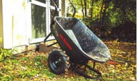
"It can carry up to 350 lbs. up a 15-degree incline and last 8 to 10 hrs. on a single charge," Cullen says. "It has a variable speed throttle that goes up to 3 mph and has forward and reverse."
