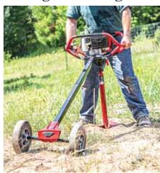
Torque reducer is built with a durable cast iron knuckle and can be flipped over when not in use to help move the auger.
