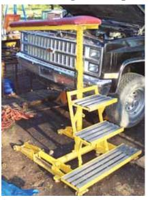
Greenwood made the base from two worn-out floor jacks while the structure was tubing, which he salvaged from packing crates and old machinery.
