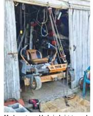
Meeks put an old chain hoist to work, hooking it to the sliding door track on an old garage. He knew the track was screwed in solid to the header over the doorway.
