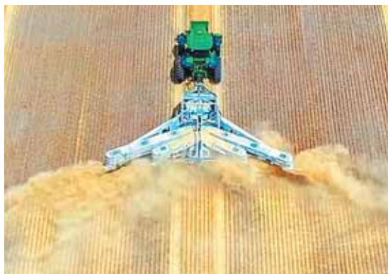
After many sets of drawings and several attempts, Wandel developed a prototype, a twin-axle 18-m. (60-ft.) unit with a pick-up to collect the straw and an elevated shredder to transport material on conveyor belts to six rotating spreaders.
