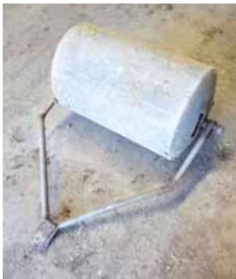
Carolla converted a pull-type roller to a 3-pt. mounted model that he uses in his landscaping and excavation business.
