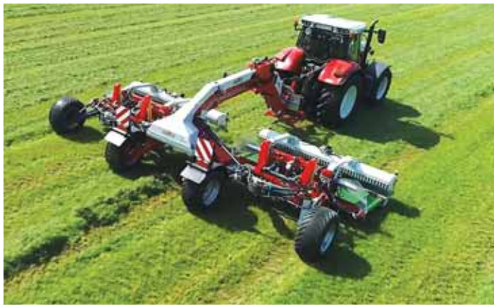
Respiro R9 Profi has a 4-wheel chassis for optimal weight distribution and four undercarriage spinning discs to effortlessly "float" the machine without bulldozing the soil.
