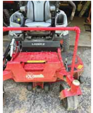
Herren's sturdy handle is made from 3/4-in. pipe.
