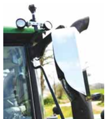
Stainless-steel mirror guards protect expensive tractor mirrors.
