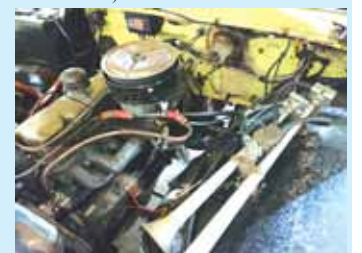
The F-250's engine is original, except for a new battery and long pipe air horns.
