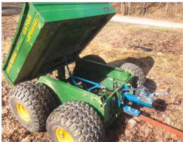
Walters set to work by cutting the trailer in half. "From there, all I needed to add was a wagon-style tongue, and I had a utility trailer."
