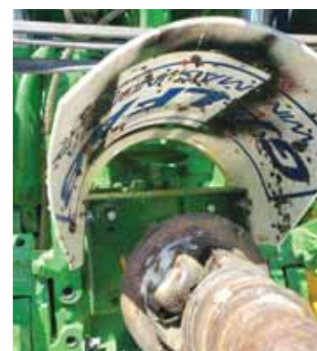
"It took me less than 5 min. to make this cover," says Pittman. "Because it's longer, it catches all of the grease that flies off the PTO shaft."
