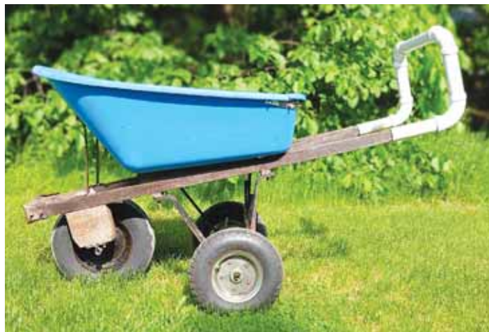
Zonies made the handles from 1 1/2-in. PVC pipe, a diameter which he found telescopes neatly over the original wooden handles.
