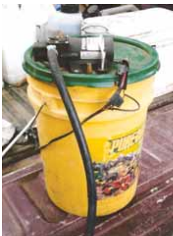
Dorris used a 35-psi pump with a 5-gal. bucket to make a handy sprayer.
