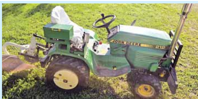
Troyer mounted a belt-driven hydraulic pump to the electric clutch intended to power a mower deck.
